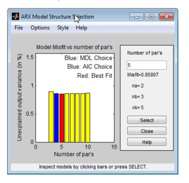
**Note** The Rissanen MDL and Akaike AIC criteria produces equivalent results and are both indicated by a blue rectangle on the plot.
