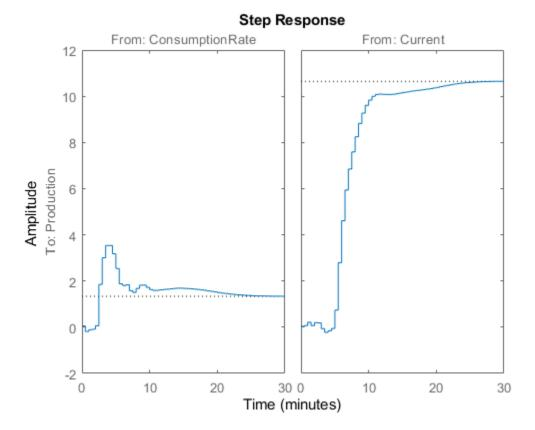
The step response for the first input/output combination suggests an overshoot, which indicates the presence of an underdamped mode (complex poles) in the physical system.
