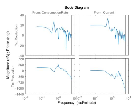
The amplitude peaks at the frequency of 0.54 rad/min, which suggests a possible resonant behavior (complex poles) for the first input-to-output combination - ConsumptionRate to Production .
