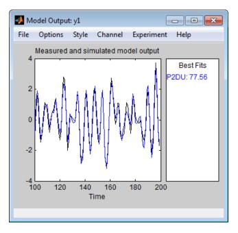
The System Identification Toolbox software uses input validation data as input to the model, and plots the simulated output on top of the output validation data. The preceding plot shows that the model output agrees well with the validation-data output.
