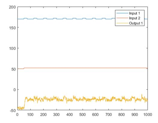
The first plot shows the first experiment, where the operator applies a pulse wave to each input to perturb it from its steady-state equilibrium.
