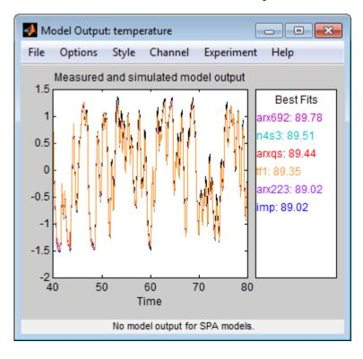
**Tip** If you closed the Model Output window, you can regenerate it by selecting the **Model output** check box in the System Identification app. If the new model does not appear on the plot, click the model icon in the System Identification app to make the model active.
