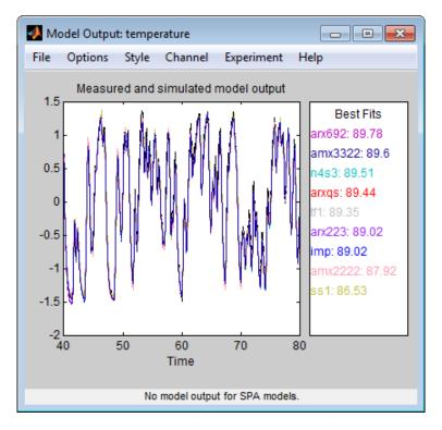
**Tip** If you closed the Model Output window, you can regenerate it by selecting the **Model output** check box in the System Identification app. If the new model does not appear on the plot, click the model icon in the System Identification app to make the model active.
