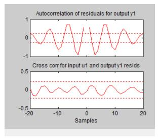
The whiteness test for P2DUe2 shows that the residuals are uncorrelated, and the independence test shows no correlation between the residuals and the inputs. These tests indicate that P2DUe2 is a good model.
