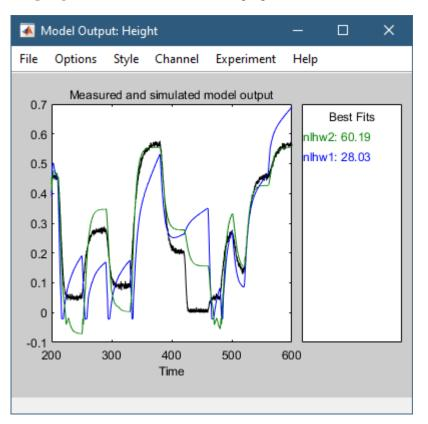
The **Best Fits** panel of the Model Output window shows the quality of the nlhw2 fit, which is an improvement over that of the model nlhw1.
