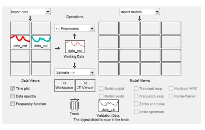
2 Drag and drop the data\_est and data\_val data sets to fill the empty rectangles, as shown in the following figure.
