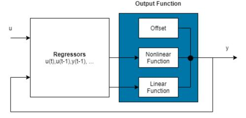
The software computes the nonlinear ARX model output *y* in two stages:
