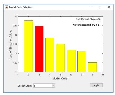
The vertical axis is a relative measure of how much each state contributes to the input/output behavior of the model (*log of singular values of the covariance matrix*). The horizontal axis corresponds to the model order n. This plot recommends n=3, indicated by a red rectangle.
