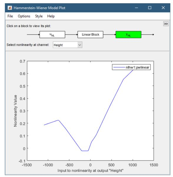
**3** Click the **Linear Block** rectangle in the top portion of the Hammerstein-Wiener Model Plot window.
