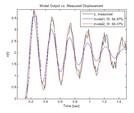
The figure indicates that model2 is better than model1 because model2 better fits the data (65% vs. 83%).
