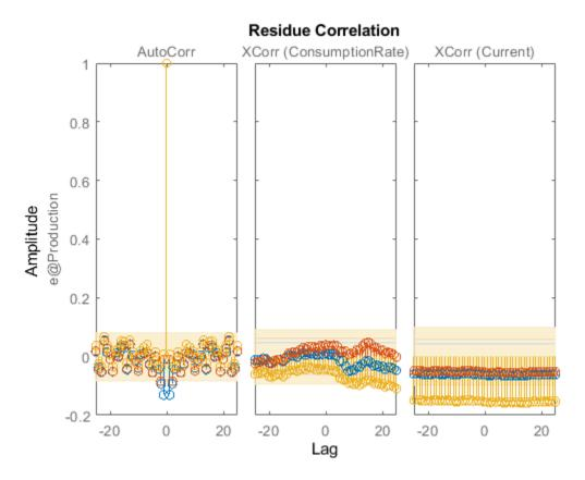
All three models simulate the output equally well and have uncorrelated residuals. Therefore, choose the ARX model because it is the simplest of the three input-output polynomial models and adequately captures the process dynamics.
