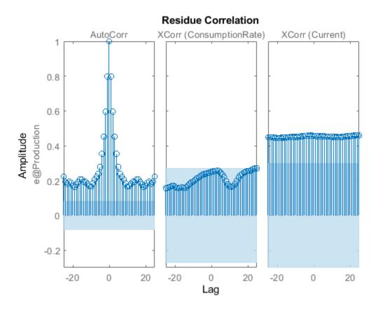
The cross-correlation between the second input and residual errors is significant. The autocorrelation plot shows values outside the confidence region and indicates that the residuals are correlated.
