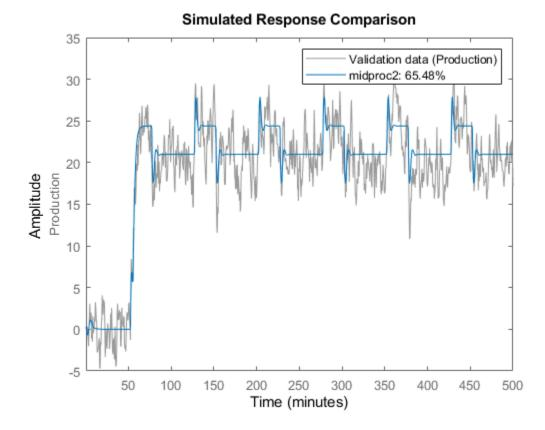
The plot shows that the model output maintains reasonable agreement with the validation-data output.
