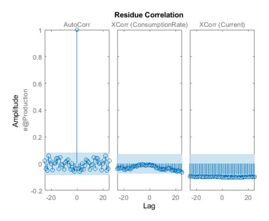
The residual plot shows that autocorrelation values are inside the confidence bounds. Thus adding a noise model produces uncorrelated residuals. This indicates a more accurate model.
