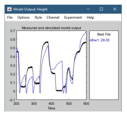
The model nlhw1 does not validate well. The fit to zv.OutputData is poor.
